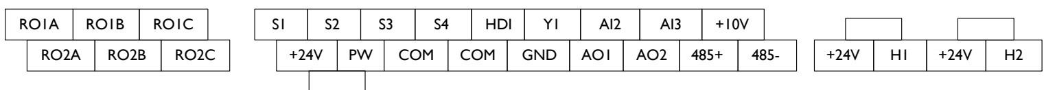
Connection terminal diagram for inverters \geq 4\text{kW}
