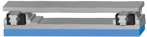
(2) Assembly of the back side of block, rail transfer
